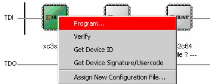
Figure 19. Loading design binary into FPGA.
