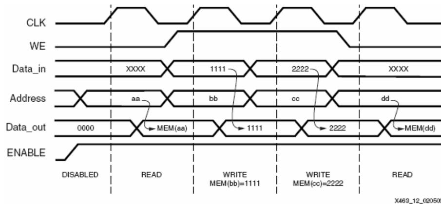
Figure 4-12: WRITE\_FIRST Mode Waveforms
