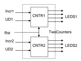
You need to detect the transitions of Incr inputs and increment/decrement the corresponding counter on the transitions of these inputs. Otherwise, it will count up/down with 50 MHz clock, which is not what we wanted.
