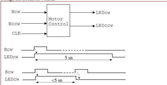
An example key-debouncer module is given with this sheet (if needed);
