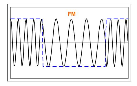
Remember that when there is only a finite number of frequency values, it is FSK. When there is only a finite number of phase values, it is called PSK.
