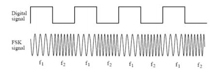
In frequency shift keying, the signals transmitted for spaces (binary zeros) and marks (binary ones) are  $s_0(t) = A \cos(2\pi f_0 t + t_0)$ ,  $0 < t \le T_b$  $s_1(t) = A \cos(2\pi f_1 t + t_0)$ ,  $0 < t \le T_b$
