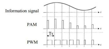
Periods (shown as Ts) of both PWM and PAM are constant. However, duration of ON state in PWM is determined by the info signal, wheras it is constant in PAM. The duration of ON state in PAM is allowed to be Ts too, that is, no OFF state.
