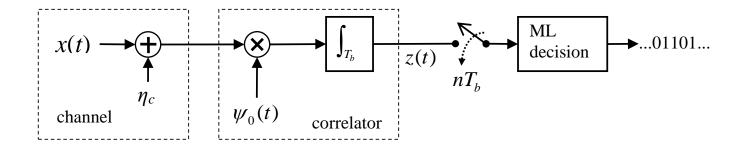
Bit rate is  $R_b=100$  kbps. Carrier frequency is  $f_c=1$  MHz. Local oscillator signal is  $\psi_0(t) = \cos(2\pi f_c t)$ . The receiver is in full synchronization with the incoming signal.
