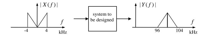
Design the system that does that using adders, multipliers and ideal filters. Give filters' cut-off frequencies.
