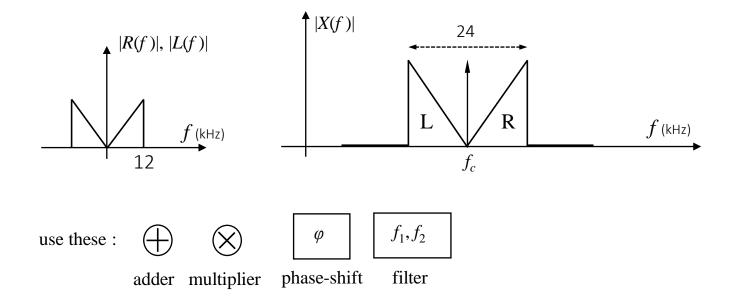
The sum of signal  $x(t) = \sin(40 \times 10^3 \pi t)$  and AWG noise  $\eta(t)$  is fed to a filter H(f) whose spectral characteristic is shown in the figure.
