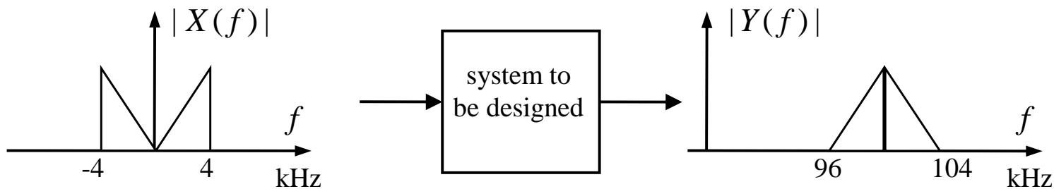
Design the system that does that using adders, multipliers and ideal filters.
