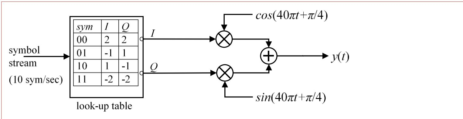
Draw  $y(t)$  when the symbol stream is  $\{00, 10, 11, 11, 01\}$ . Do not forget the axis names and scale info (tick labels) on the graph.
