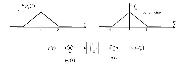
Calculate the probability of decision error  $p_{e^*}$ , assuming that the system is in full synchronization, symbol transmission probabilities are equal and the channel has no ISI (intersymbol interference)
