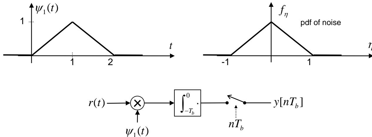
Calculate the probability of decision error  $p_e$ , assuming that the system is in full synchronization, symbol transmission probabilities are equal and the channel has no ISI (intersymbol interference)
