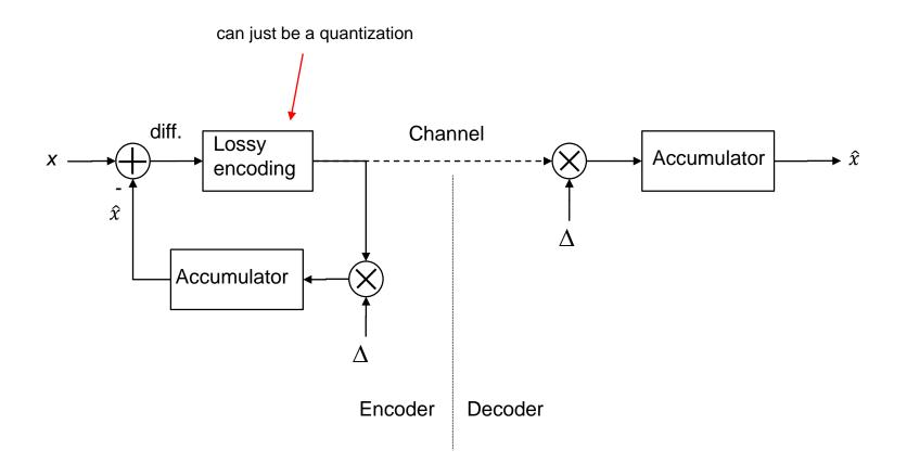
Quantization can be as simple as single bit representing + or - differences
