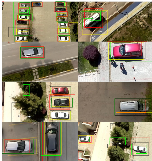
Fig. 6: Performances of classifiers on test images are represented as: YOLOv2 – Red, YOLO Tiny – Yellow, EPCC with 8 orientations – Black, EPCC with 4 orientations – Green rectangles.
