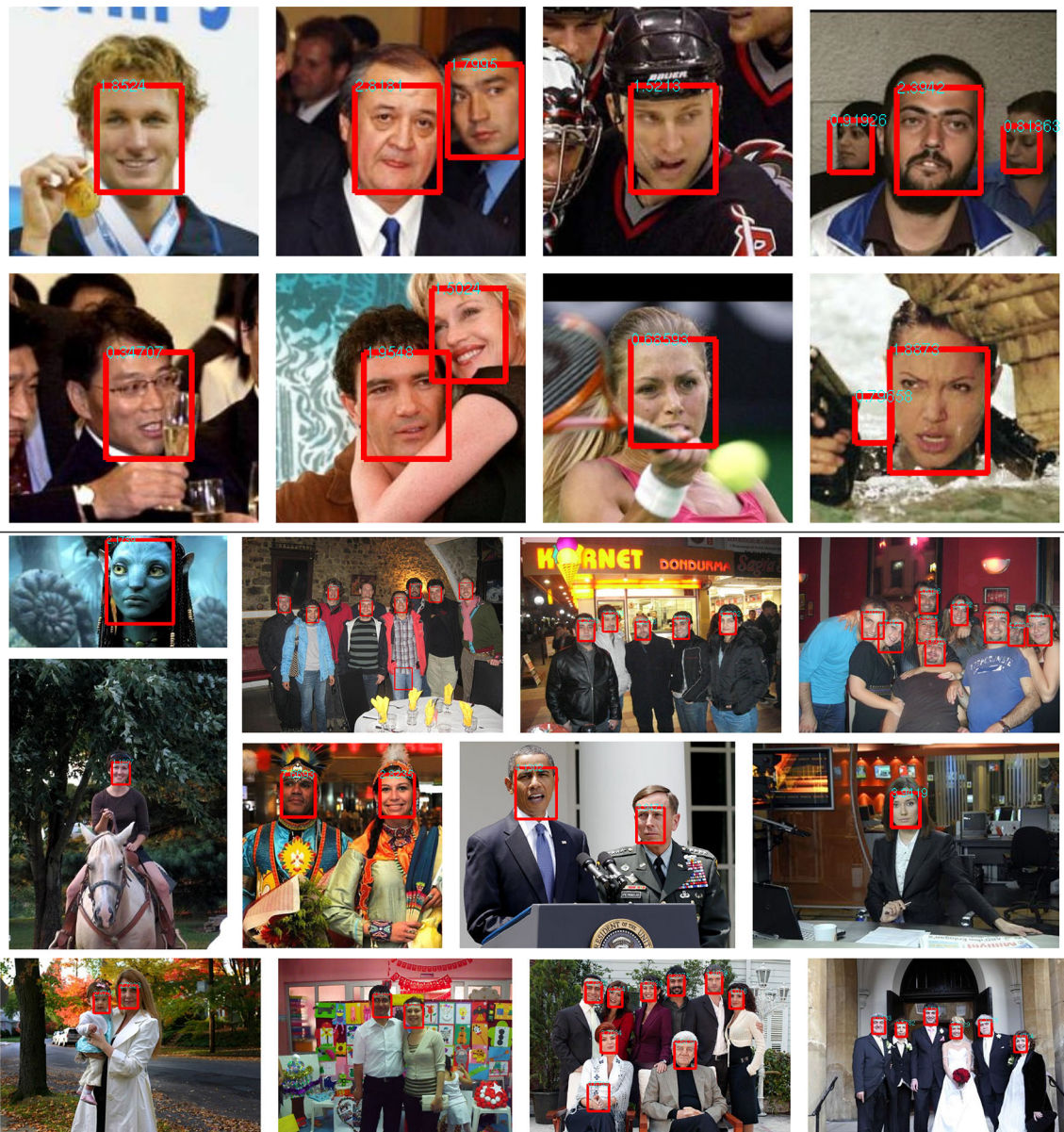
Fig. 2 Some examples of the output of our face detection cascade on images from the Labeled Faces in the Wild ( top ) and ESOGU Faces ( bottom ) datasets. Most of the faces are correctly detected, but there are a few missed detections and false positives
